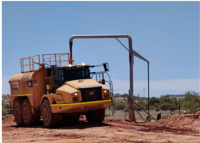
Three bores provide water for construction which is pumped and stored in turkey nests. Water trucks provide water for dust suppression, materials conditioning and compaction.
