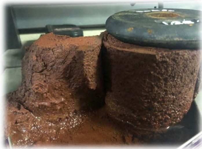
**Figure 2: After 90mins the untreated sample fell apart, the Polycom sample was still within tolerance 24hrs later**
